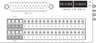
ON Not connected to a monitor (Normal) OFF Connected to a monitor (Looped)
